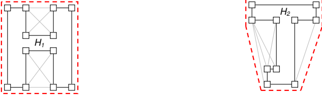
Fig. 2. Illustration of local visibility graphs for holes H_1 and H_2 . Polygons with dotted lines represent the convex hulls of the holes. In LVG-G, edges between two VON nodes in different holes are not considered.
